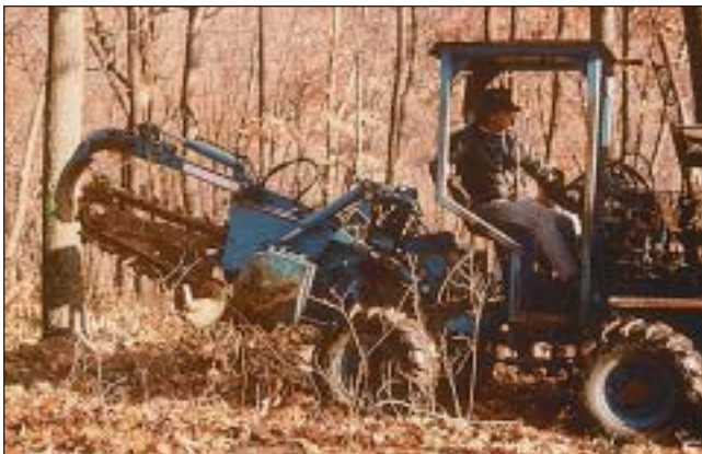
A trencher is a rubber-tired vehicle with a digging chain attached to the back. The chain moves along a boom, digging a trench and breaking root grafts as it is pulled through the soil.
